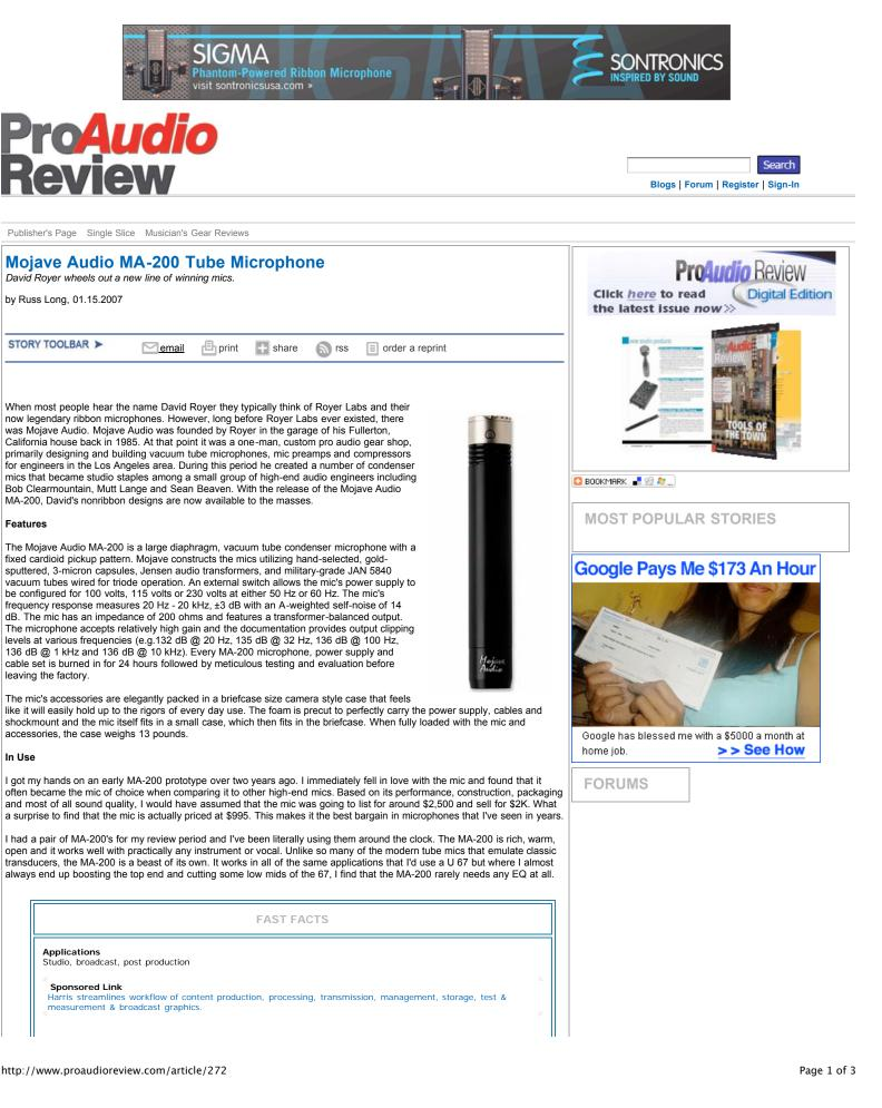
Key Features Cardioid pattern; 1-inch gold sputtered 3-micron diaphragm; tube electronics featuring military-grade JAN 5840 vacuum tubes; Jensen transformer
