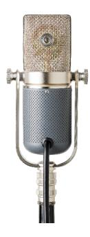
The MA-37 features a unique mechanical approach, developed by RCA in the 1930s and adapted by Sony, to achieving a choice between cardioid and omnidirectional polar patterns – an adjustable tuned acoustic chamber. To change the pattern selection from cardioid (C) to omni (O), insert a small flat-head screwdriver into the slot and rotate clockwise approximately 90 degrees. It is perfectly acceptable to stop anywhere between C and O in order to achieve a hyper-cardioid polar pattern.
